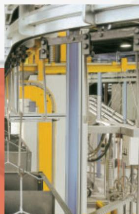
Inlet for workpieces of a powder coating booth
